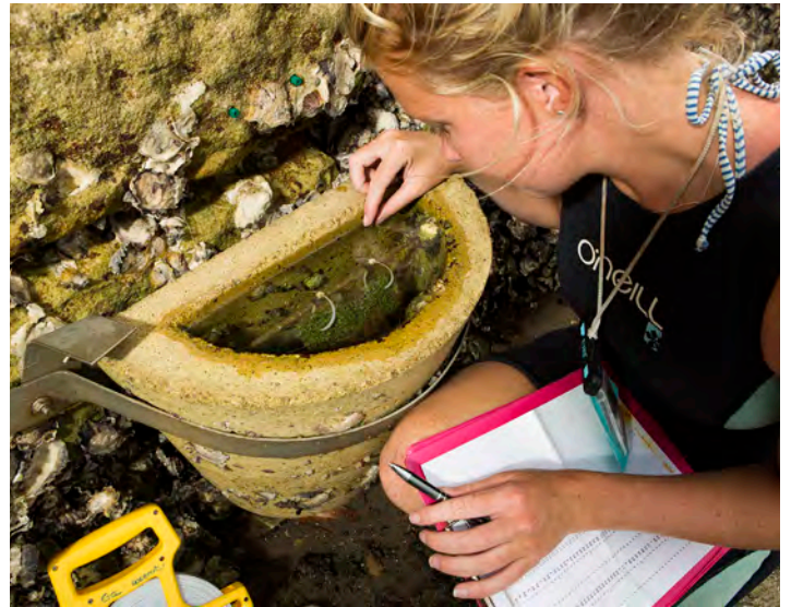
Along the Glebe foreshore, seawall pots have been installed as a trial and are attracting many varieties of species
